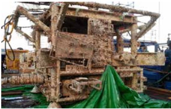
*Puffin subsea manifold on deck, with dense marine growth clearly evident.*
